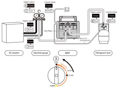
Connect the hoses tight as shown in the diagram above.
