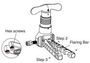
4. Place the tubing depth stopper at the right size. Insert copper tubing up to the tubing depth stopper.
