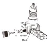
7. Using ¼" hex drill bit, insert it to the hex socket on the expander end. With the drill set for clockwise turning, start the drill and continue until the clutch engages (clicking).
