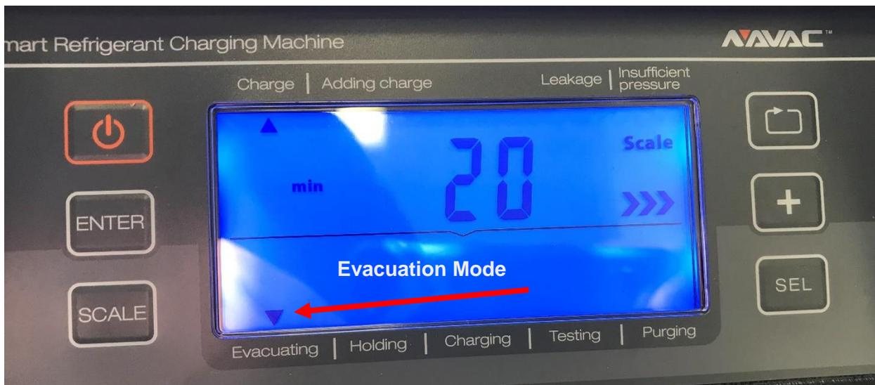
4. It will then enter a "Holding" mode for 2 minutes. If within that time, the vacuum change is within the acceptable level, it will advance to Charging Mode.
